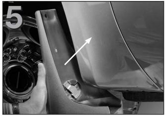
Position the smooth surfaced portion of the MudFlap so that it contours firmly against the fender as shown. **IMPORTANT** - Ensure that the QuickTurn<sup>™</sup> fastener remains in the fully unlocked position during this step.
