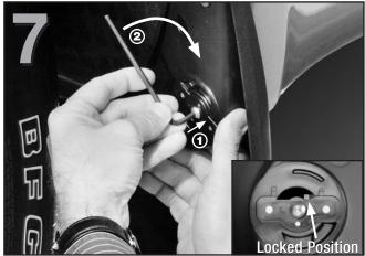
First ensure that the QuickTurn<sup>™</sup> fastener is positioned properly by pressing in the direction indicated by arrow 1. Then, hand tighten the QuickTurn<sup>™</sup> fastener (arrow 2). Verify that the QuickTurn<sup>™</sup> fastener is in the fully locked position.
