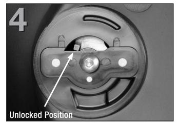
Identify the driver's side MudFlap by locating the "LH" mark located centrally in the recessed cavity on the tire side of the MudFlap. Ensure that the QuickTurn<sup>™</sup> fastener is in the fully unlocked position using the Allen wrench provided.
