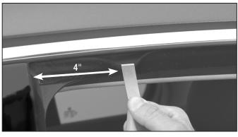
Pull down the weather-strip in the front location, approximately 4" from the front. Then, push clip in, and replace weather-strip.
