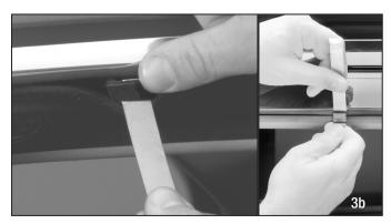
Continue pulling down the weather-strip to insert a channel clip. Small/short channel clips can be easily installed by inserting the middle flat portion upwards into the channel first. Longer channel clips can be installed by using the installation tool shown in Picture 3h
