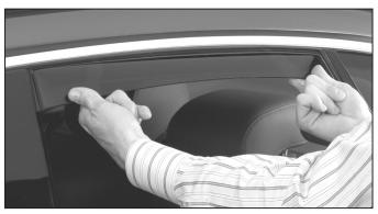
Inspect deflector to ensure that it is fully inserted into the window channel. The channel clips should match the contour on the backside of the deflector. Next, close your window fully and press firmly against weather-strip from front to rear.
