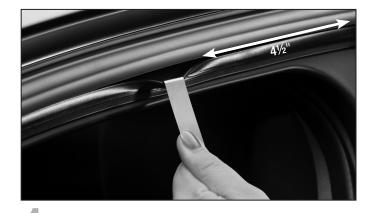
Make sure that the window is clean and dry. Then pull down the weather stripping in the first position, which is approximately 4½" from the rear
