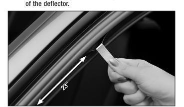
Pull down the weather stripping in the second position, which is approximately 23" from the front mirror.
