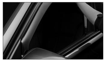
Inspect the deflector to ensure that it is fully inserted into the window channel. Slowly and carefully, close your window fully and press firmly against weather strip from front to rear without engaging auto-up feature.
