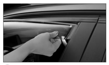
Bow the deflector outward to insert the rear flange into the window channel. Making sure the window gasket is not folded over.
