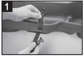
Install the safety strap through the slot on the rear.
