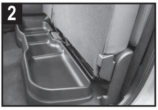
Position the Under Seat Storage under the backseat as shown.
