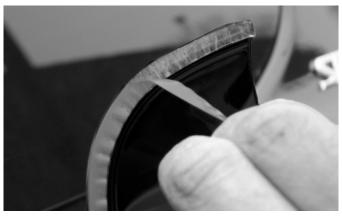
Remove the red tape backing from one end of the deflector to the other. Avoid touching the adhesive to keep it clean.
