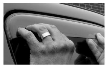
Carefully align deflector along the top of the window.
