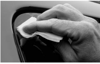
1 Dry fit deflector on window before installing. Clean the installation area of the glass with the included alcohol wipe, allow to dry. NOTE: Glass must be cleaned for the Side Window Deflector to attach properly.
