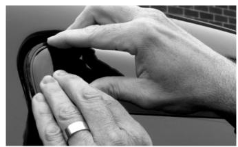
Press and hold deflector firmly in place for at least 30 seconds to ensure proper attachment to the window. IMPORTANT: Avoid rain or washing the vehicle for at least 72 hours to allow adhesion to set.
