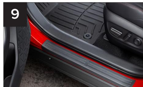
**9** Congratulations on installing your WeatherTech SillProtectors! Your SillProtectors will be fully bonded within 24 hours. Do not wash your vehicle for 72 hours after installation.
