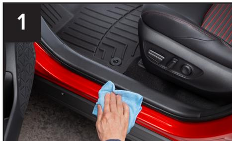
**1** Wash the door sills of your vehicle and completely dry with a clean cloth. It is important that the door sills remain completely dry and free of any dirt and debris throughout the installation process.
