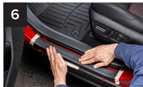
**6** Carefully place the SillProtector back into position within the outlined masking tape on your door sill. Remove the masking tape after SillProtector is in place.
