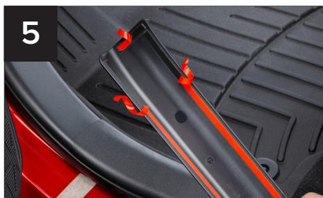
**5** Prepare for installation by peeling back the adhesive liner from each section on the underside of the SillProtector. Fold the adhesive liners back far enough to create pull tabs.
