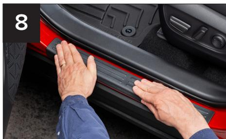
**8** Using the palm of your hand, apply additional pressure from the center out, pressing down firmly along all the adhesive lined edges to ensure proper adhesion.
