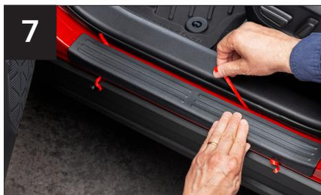
**7** Remove the adhesive liner. Grasp the exposed portion of the adhesive liner and pull gently with one hand while applying light, even pressure to the SillProtector with your opposite hand. Repeat this step until all adhesive liner has been removed.
