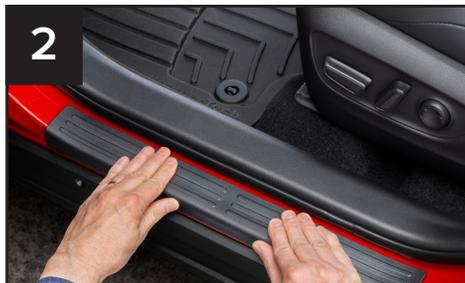
**2** Place SillProtector on door sill for a trial fit. Make sure you are using the character lines of your door sill to match with the SillProtector.
