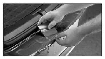
Continue to use the squeegee to work bubbles toward the edges until eliminated, aggressive use of the squeegee can damage the film.
