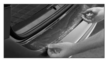
Using the top edge as a guide and centering the film as best you can, apply the template to the trunk ledge. Starting from the top and working down, use the squeegee to apply slow, gentle strokes to force the solution and air bubbles down and out.
