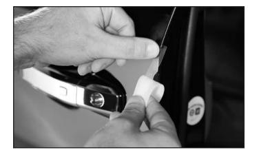
Locate desired starting point for the film; body lines are an excellent guide. Peel back 3-4" of film from backing. Apply half the film width on the front edge and firmly press it down. Continue application until the end of film is reached.
