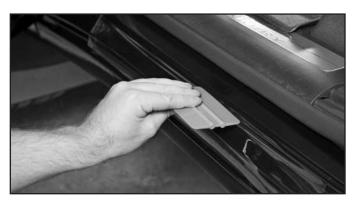
Use the squeegee as needed to finish the application, aggressive use of the squeegee can damage the film.
