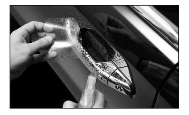
Spray alcohol solution on the door cup area, fingers and protection film before and as the film is removed from the backing.
