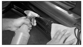
Thoroughly clean all areas with the alcohol solution to remove any dirt, debris, grease or oil. Dry with a clean, lint-free cloth.
