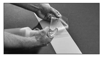
Locate desired spot for film application. Spray soap solution on your fingers and protection film as you remove it from the backing.
