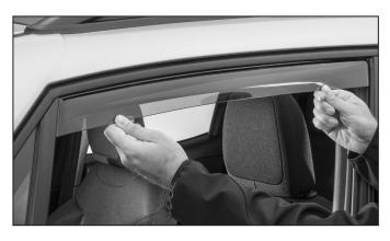
Inspect deflector to ensure that it is fully inserted into the window channel. The channel clips should match the contour on the backside of the deflector. Next, close your window fully and press firmly against weatherstripping from front to rear.
