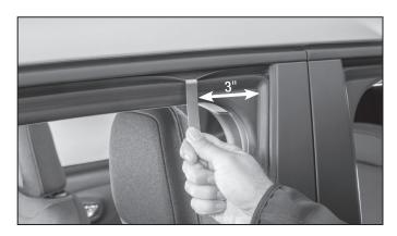
Make sure that the window is clean and dry. Then pull down the weatherstripping in the first position, which is approximately 3" from the rear of the deflector.
