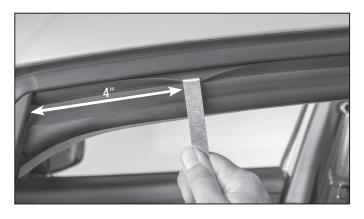
Pull down the weatherstripping in the second position, which is approximately 4" from the front. Then, push clip in and replace weatherstripping.
