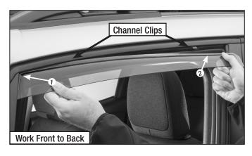
Working front to back, fully insert machined flange of deflector into window opening over the clips, while pressing inward against channel clips. If the deflector has hemispherical notches, center the clips under them prior to deflector installation.
