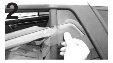
Carefully insert the rear deflector's rear flange between the rubber seal and the window. This can be a tight fit on some vehicles, and it is usually beneficial to loosen the rubber in this area with something flat. DO NOT use a knife or other sharp object, as this can cause injury to you and your vehicle!
