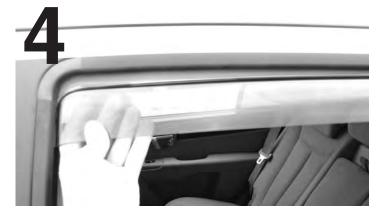
Continue to press upward on the deflector until it is fully seated along the edge of the window seals.
