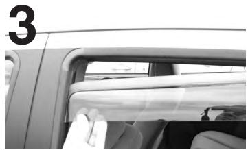
Insert the deflector's front flange into the window channel and slide the deflector upwards while taking care to guide the deflector's top flange into the window channel at the same time.
