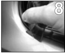
Complete installation by lifting the end of deflector onto retention clip.
