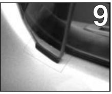
Push forward on deflector until it is fully inserted into the window channel. Slowly and carefully close the window for the first time.
