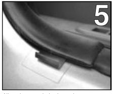
Allow the curved plastic portion to return to its original location, covering the retention clip.
