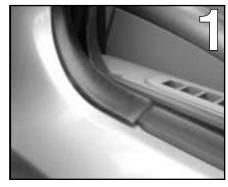
Open drivers window completely. Note curved plastic portion at forward base of window opening.
