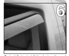
Begin deflector installation by inserting end of deflector into the window opening at the rear end of the door. (upper right hand corner)
