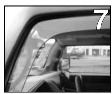
Continue inserting the deflector into the window channel from rear to front, working toward tip, or leading edge of deflector.
