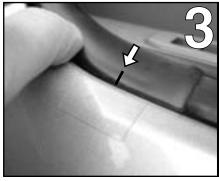
Install the 3M® paint protection film on the doorskin, adjacent to the curved plastic and center the film at the 1 1/8" mark.
