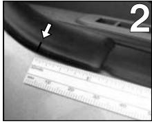
Measure a point 1 1/8" from the point where the curved plastic begins, and mark with a felt tip pen.
