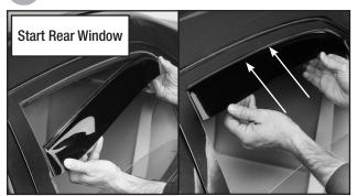
Be sure to remove adhesive backing before installation (if supplied). Slide upward into place, then gently pull outward to set the deflector.
