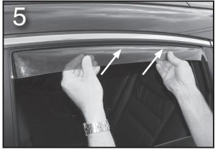
Gently tug the part outward to ensure that the deflector is seated properly. Slowly and carefully roll up the window.
