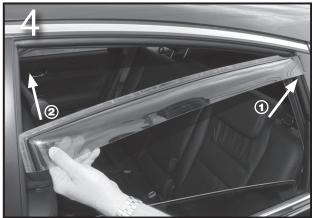
Put the rear edge of the deflector into the clip first. Then insert the front flange into the window channel. Push the deflector upwards until the top flange is fully inserted into the window channel.
