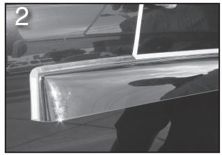
Remove the tape backing from the front and upper flanges. Avoid touching the adhesive.
