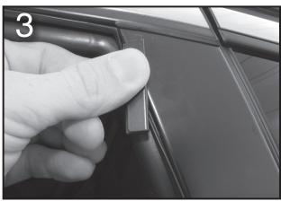
Insert one of the clips between the rubber gasket and the black plastic that forms the rear edge of the window.
