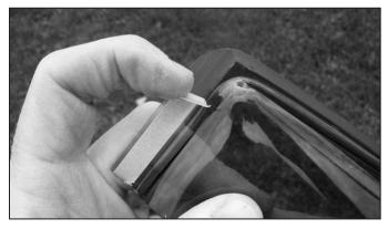
Remove the protective film from the adhesive attached to the deflector.
