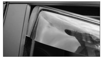
Begin the deflector installation by inserting the machined flange of the deflector into the front-end of the window opening. Install from front to rear, slipping rear flange of deflector between clip and window frame. The clip will apply outward pressure against deflector to aid retention. Repeat Steps 1-6 for the passenger side installation.
