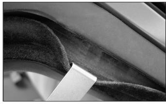
Using the small "hook end" of the installation tool, carefully pull-down the inner rubber weatherstrip material at the location determined in Step 1.
