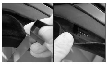
Place the retention clip into the exposed opening of the rubber window channel as shown, with the curved portion facing outward. Push it up, and fully into the window channel (you may push it with the installation tool if necessary).
