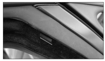
Push the weatherstrip molding back into place as shown in the photo. Only a small portion of the metal retainer clip will be exposed.
