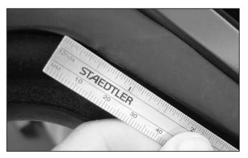
To install retention clip, measure-down approximately 1" (25mm) from rear corner of window opening. Mark this location with a felt-tipped pen or pencil.
