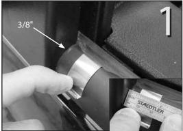
Open driver-side window. Hang a clip on the rubber belt molding in the outer molding and dew wiper as shown. Some folding of the outer molding is normal and necessary for proper fitment.
