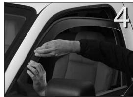
The rear edge of the deflector should be pulled down slightly (exagger ated in the photo). Pull the deflector down and tuck the flange into the window channel working from front to back.
