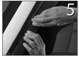
Continue tucking the flange into the window channel until it is resting in the window chan nel along its entire length.
