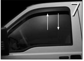
Slowly inch the window upward until the window is completely closed. Repeat this 5 times. It is a good idea to leave the window completely closed for several hours after installation to ensure perfect fit.
