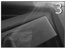
Insert the deflec tor's rear flange into the window channel.
