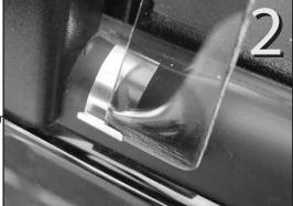
Place the bottom of the driver's side de flector into the clip and slide it forward until it seats firmly against the mirror bracket. Ensure that the deflector's front flange is inserted into the window channel.
