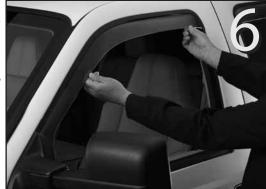
Gently pull outward to seat the deflec tor and ensure that none of the window rubber has been folded inward while inserting the flange.
