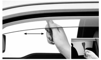
Insert flange seating tool into the window channel and run it back and forth fully to seat the deflector.
