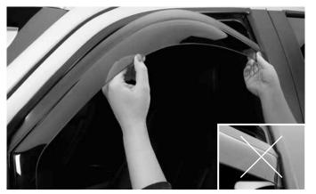
**5** Bow the deflector outward to slip the rear flange into the window channel, making sure the window gasket is not folded over.
