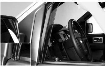
4 Insert the front of the deflector as shown; ensure edge rests on the top of the outer window sill.
