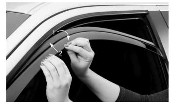
6 Starting from the front of the deflector, begin tucking the flange into the window channel.
