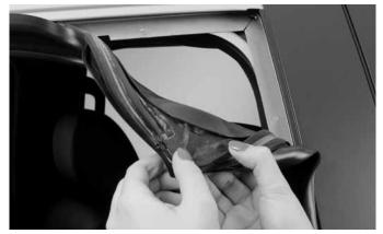
**2** Pull down the weatherstrip from the upper right corner of the window opening as shown.
