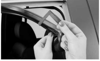
**3** Remove and discard the L-shaped foam pad inside the weatherstrip, then push the weatherstrip back into place.
