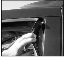
Open drivers window. Grasp rubber window gasket with your fore finger and thumb, and peel back to expose window frame.
