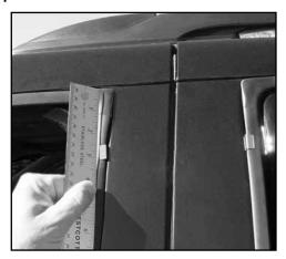
With window frame exposed, insert clip onto vertical part of window frame, just below curved portion in corner. Clip should be placed approximately 2½ inches from top of rubber gasket (over spot weld).
