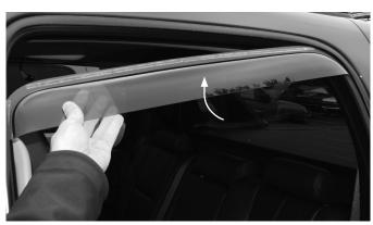
Slide the front of the deflector upward until all the deflector's edges are fully seated into the window channel.
