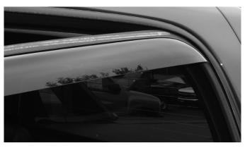
Insert the rear edge of the deflector into the window channel as shown. Next, align the front edge of the deflector in line with the window channel.
