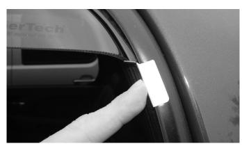
Slide the retention clip onto the outer window trim as shown. Ensure that the clip is touching the bottom edge of the deflector. Note that the clips included with your kit are black.
