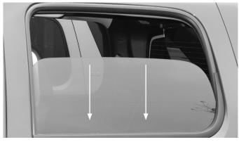
Start with the left hand side of your clean vehicle. Completely roll down the rear windows. Remove the adhesive backing from the drivers side part.
