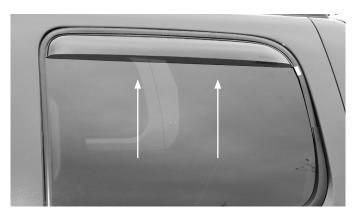
Carefully roll up the window up. To complete installation, repeat steps 1-5 on the passenger side.
