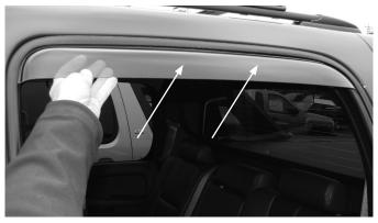
Gently pull outward along the full length of the deflector to properly seat the adhesive.
