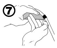
Grasp the rear-end of the deflector firmly with both hands and bow the deflector *just* until you can insert the tip of the rear retainer into the hole on the deflector.
