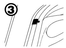
Push the weatherstrip molding back into place as shown.
