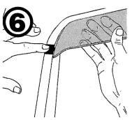
Begin the deflector installation by inserting the machined flange of the deflector into the front-end of the window opening, while at the same time, inserting the tip of the retaining clip into the small hole of the deflector.
