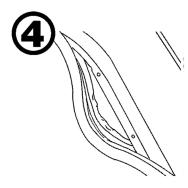
Peel back the weatherstrip molding in the *upper right-hand corner* of the driver's window opening and insert the rear retainer onto the exposed metal flange of the window frame.
