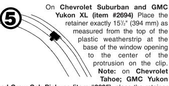
and Crew Cab Pickups (item #2695), place the retainer exactly 15% (384 mm) as measured from the top of the plastic weatherstrip at the base of the window opening to the center of the protrusion on the clip. Push the weatherstrip molding back into place as shown
