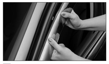
Starting with the front of the deflector, begin tucking the flange into the window channel while pressing inward against the channel clips. Be sure to tuck the flange between weather stripping and the channel clip.
