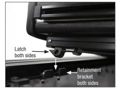
C. Unhook storage clips at front of cover and unfold middle panel towards tailgate. Hooks on middle panel will automatically engage middle catch on each side.
