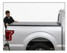
B. Fold middle panel on top of front panel.
