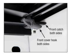
B. With cover hooks engaged underneath front catches, lower cover and engage latch in retainment bracket on each side.
