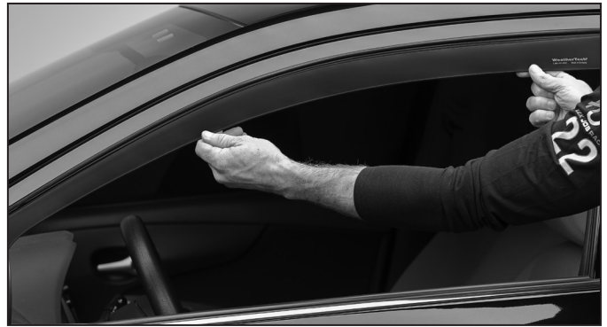
6 Carefully pull outward on the deflector.
