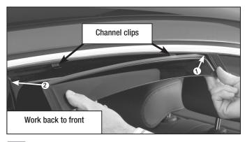
Working back to front, fully insert machined flange of deflector into window opening over the clips, while pressing inward against channel clips. If the deflector has hemispherical notches, center the clips under them prior to deflector installation.
