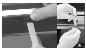
Continue pulling down the weather-strip to insert a channel clip. Small/short channel clips can be easily installed by inserting the middle flat portion upwards into the channel first. Longer channel clips can be installed by using the installation tool shown in Picture 3b.
