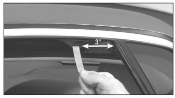
Make sure that the window is clean and dry. Then, pull down the weather-strip with the provided tool approximately 3" from the rear edge.
