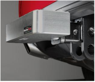
Align the BumpStep<sup>™</sup> to the deepest hole position allowed by your receiver.
