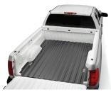
Place UnderLiner<sup>™</sup> in the bed of your truck. Align contours and cutouts for the wheel wells to allow UnderLiner<sup>™</sup> to lay flat and smooth.
