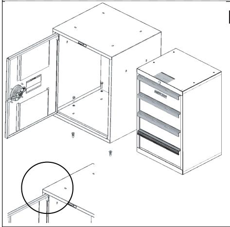
Place a drop of oil on the black oxide bolt before assembling as shown on right. Place the Blind Fastener in the hole and use a 7/16 wrench to tighten black hex bolt until the Blind Fastener is fully seated. When setting black hex bolt, it will start out hard. As the Blind Fastener "bulbs" out it will get easier, until it bottoms out or sets. Make sure the Blind Fastener and Installation Tool do not turn during installation.
