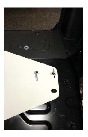
**STEP 12.** Secure the Front and Rear shelving units using (4) M6-1.0 x 16mm bolts, (4) flat washers, and (4) M6-1.0 lock nuts through the previously installed Mid Bracket and 36" Wide Shelf Mounting Foot.
