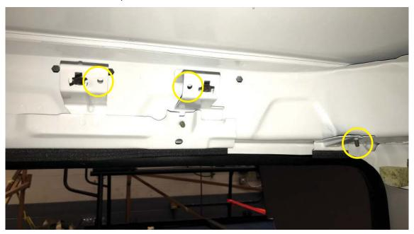
**STEP 9.** Remove the OEM plastic caps from the floor mounting points near the front of the floor. Note that they are used to install WEATHER GUARD® Bulkhead 96112-3-01 or 96512-3-01. The outer most mounting point will be used to install the 28" shelving unit. Be sure to install the bulkhead prior to shelving installation when using WEATHER GUARD® Bulkhead 96112-3-01 or 96512-3-01.
