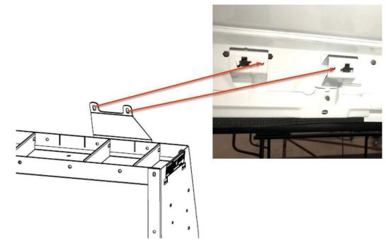
STEP 14. Loosely assemble L-bracket, 1.25" Spacer, and a Mounting Strap using (2) washers, M6-1.0 x 50mm bolt, and a M6-1.0 lock nut. L-bracket and Mounting Strap are supplied with the shelving unit. Attach the assembly to the threaded stud using a washer and a M6-1.0 Lock Nut. Attach the Mounting Strap to the end panel using M6-1.0 x 16 mm bolt, flat washers, and M6-1.0 lock nut.
