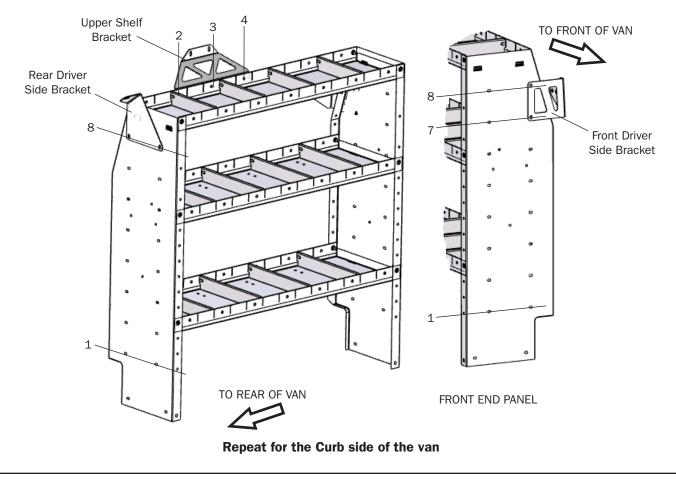
**STEP 5.** Place the Driver Side shelf unit in the van and fit it between the front and rear mounting feet. Alight the brackets on the end panels and the shelf with the mounting holes in the van.
