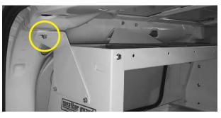
**STEP 6.** Check for shelf unit alignment and straightness and after making any adjustments, tighten the mounting hardware.
