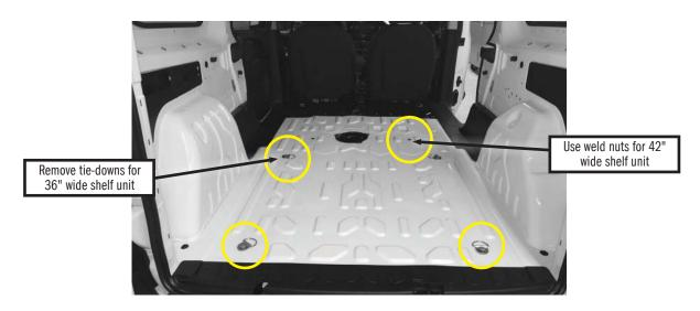
STEP 2. Determine if you will be installing 36" wide or 42" wide shelving and select the appropriate mounting feet. Starting at the rear of the van, install a Mounting Foot to the van floor using (1) M8-1.25 x 40mm bolt and (1) 12.7mm thick floor spacer. Use the 13mm socket and driver to loosely attach the mounting foot. Do not completely tighten at this time, allowing the foot to pivot about the mounting bolt. Repeat with the Curb Side Front Mounting Foot.
