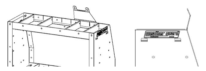
STEP 11. Install the Front Mounting Foot the 28" shelf using (2) M6-1.0 x 16mm bolts, (2) flat washers, and (2) M6-1.0 and place the 28" shelf alongside 36" Rear Shelving unit. Front Mounting Foot will align to the outer most weld nut on the floor. Use a spacer and M8-1.25 x 40mm bolt to secure the Front Mounting Foot to the floor.
