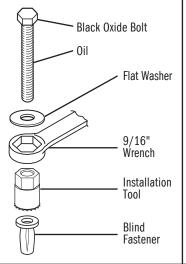
Place a drop of oil on the black oxide bolt before assembling as shown on right. Place the Blind Fastener in the hole and use a 10mm socket and driver to tighten the black hex bolt until the blind fastener is fully sealed.
