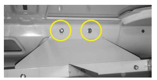
Using (1) M6-1.0 x 16mm bolt, attach the Rear Driver Side bracket to the M6 blind fastener installed in Step 3 with the 10 mm socket and wrench. Do not completely tighten yet.
