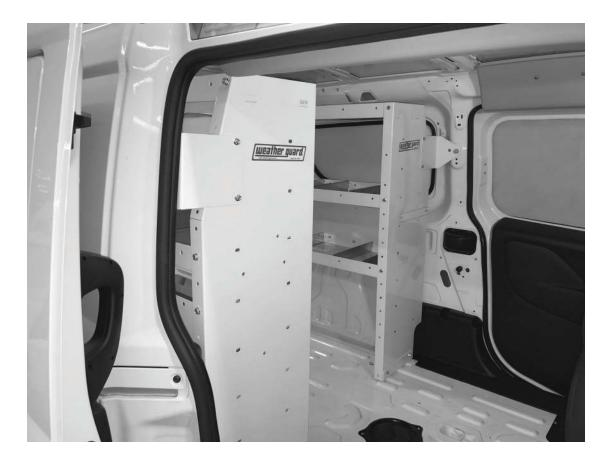
**STEP 7.** The following steps will apply to driver side front shelf installation. Passenger side installation will mirror the driver side installation using the passenger side specific bracket and a common front mounting foot.
