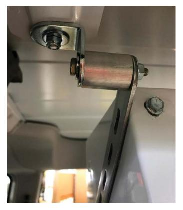
STEP 15. Check for shelf unit alignment and straightness and after making any adjustments. Tighten the M6 bolts and lock nuts to 10 ft-lbs. using the 10 mm socket and the torque wrench. Tighten the M8 bolts to 15 ft-lbs. using the 13 mm socket and the torque wrench. Tighten the 7/16" bolts to 26 ft-lbs using a 5/8" socket and the torque wrench.
