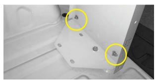
Using (1)  $7/16-20 \times 3/4$ " bolt and (1) 7/16 flat washer, attach the bracket on the front end panel to the van with a 5/8" socket and driver. Do not completely tighten yet.
