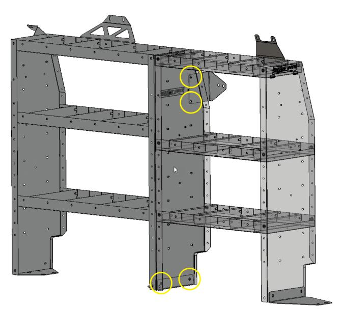
**STEP 13.** Secure the Front Upper Bracket using (2) M6-1.0 x 16 mm bolts, (2) flat washers, and (2) M6-1.0 lock nuts.
