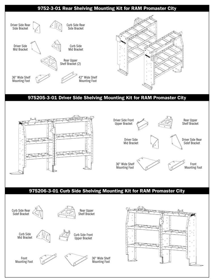
Using these mounting brackets you will be able to install 36" wide or 42" wide rear shelving units in a RAM Promaster City using pre-existing weld nuts and mounting holes when installing 9752-3-01. WEATHER GUARD® van shelving and accessories provide flexibility in customizing the storage space for the needs of tradesmen and professionals.
