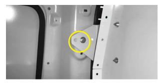
Using (2) M6-1.0 x 16mm bolts, attach the Upper Shelf bracket to M6 blind fasteners installed in Step 3 with the 10 mm socket and wrench. Do not completely tighten yet.
