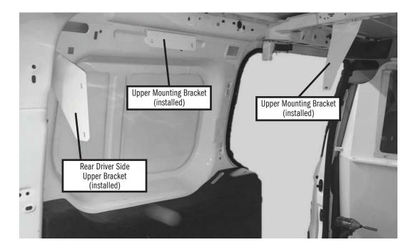
**STEP 5.** Attach the Rear Mounting Bracket to the end panels facing the rear door using (2) M6-1.0 x 16mm bolts, (2) flat washers, and (2) M6 Lock Nuts.
