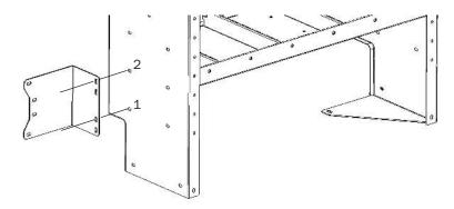
**STEP 6.** Place the 36" wide shelf unit in the van and fit it to the mounting brackets and mounting foot.
