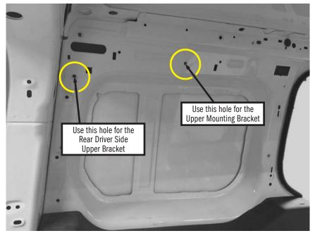
Attach one Upper Mounting Bracket to the weld nut in the center of the side panel using (1) M6-1.0 x 16mm bolt and (1) flat washer with a 10mm socket and driver.
