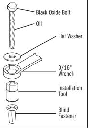
Place a drop of oil on the black oxide bolt before assembling as shown on right. Place the Blind Fastener in the hole and use a 10mm socket and driver to
