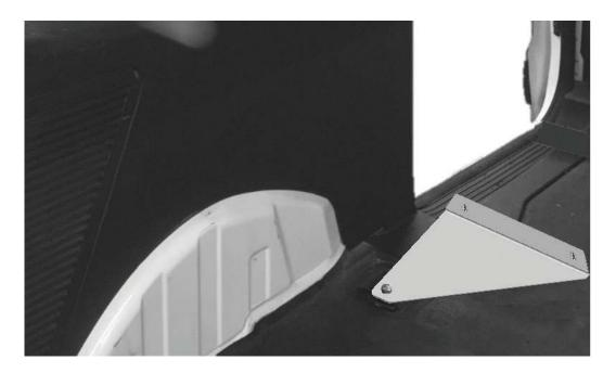
**STEP 3.** The Driver Side Mid Upper Bracket for the 36" wide shelf units attach to the van roof bow with two blind fasteners. Referring to the picture below, locate the holes in the roof bow for the blind fastener. Follow the instructions below and install the M6 blind fastener in these holes on both the driver and curb sides as well when installing 9751-3-01.
