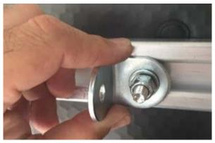
STEP 15. Install the end strap to the L-bracket using 1/4-20 x 3/4" bolt, washer, and nylon lock nut using 7/16" wrench and socket. Position the strap such that it is inline with the end panel. Align the end strap to one of the holes on the end panel and secure it using 1/4-20 x 3/4" bolt, washer, and nylon lock nut. Make sure all components are aligned and tighten.
