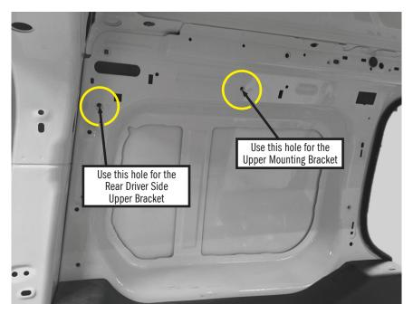
Attach one Upper Mounting Bracket to the weld nut in the center of the side panel using  $(1) M6-1.0 \times 16 mm$  bolt and (1) flat washer with a 10 mm socket and driver.
