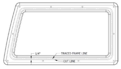
**STEP 7.** Use #10-24 screws, washers, and nylon lock nuts to attach the window panel and frames to the bulkhead panel. The window panel will sit within the recess (on the cargo side) of the bulkhead with a frame on the outside of the window panel sandwiching it against the bulkhead. The other frame will be on the embossed/cab side of the bulkhead. Tighten to 23 in-lbs.
