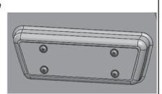
**STEP 3.1** From the Cab Side, use (4) 1/4"-20 screws and washers through the Reinforcement Bracket to attach the Accessory Panel. Tighten to 76 in-lbs.
