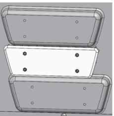
**STEP 2.2** Place and hold the Accessory Panel in line with the drilled holes on the Cab Side.
