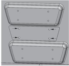
**STEP 1.2** Using a 5/16" drill bit, use the Reinforcement Bracket as a template to drill 4 holes in the desired Panel location.
