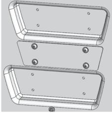
**STEP 3.2** From the Cargo Side, use (4) 1/4"-20 screws and washers through the Reinforcement Bracket to attach the Accessory Panel. Tighten to 76 in-lbs.
