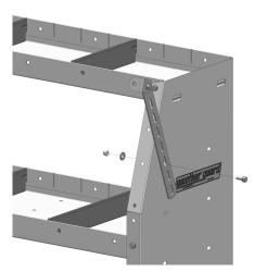
It is important to make sure that the mounting straps are attached on the end panels perpendicular to the van walls. The mounting strap needs to be bolted at two points at minimum where the strap and the end panel meets. Attach the mounting strap to end panel using a exisinting obround hole such that the strap can pivot and is long enough to reach the van wall. Use a  $1/4-20 \times 3/4$ " bolt with washer and a nylon lock nut but do not tighten at this time.
