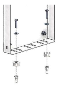
STEP 8. Finish installing the mounting straps by aligning then drilling additional hole for the second attachment point mentioned in STEP 3. Use a 1/4-20 x 3/4" bolt with washer and a nylon lock nut. Mounting straps can be trimmed or bent to get the best fit to the inside wall of the van.
