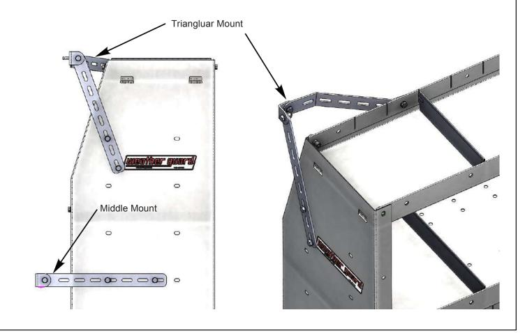
STEP 9. Verify the wall mounting locations and install blind fasteners. Existing holes may be used to install blind fasteners if they are located near the mounting straps. If not, they may still be used for ADDITIONAL mounting points using extra mounting straps. We recommend using two mounting angles on the strap joining two shelf units. One mounting foot can be shared between two shelf units.
