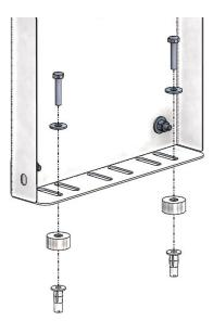
**STEP 8.** Finish installing the mounting straps by aligning then drilling additional hole for the second attachment point mentioned in **STEP 3**. Use a 1/4-20 x 3/4" bolt with washer and a nylon lock nut. Mounting straps can be trimmed or bent to get the best fit to the inside wall of the van.
