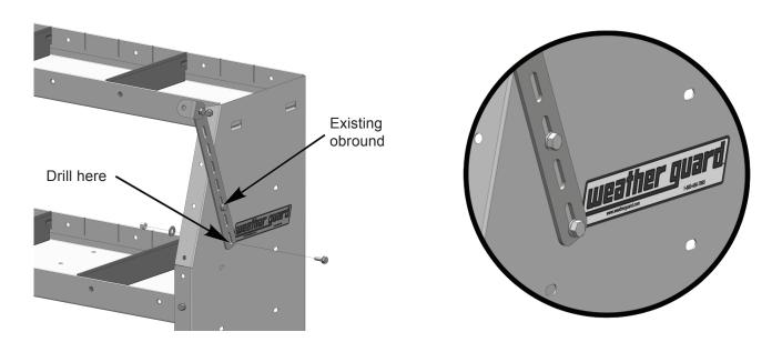
Install middle mounting point when possible. You can bend the mounting strap to create a triangular mounting to strengthen the shelf unit.
