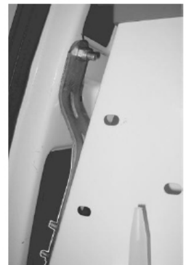
Bent Mounting Strap attached to inside edge of End Panel.
