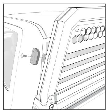
Insert square nut into slot. Loosely fasten attachment point using screw provided.
