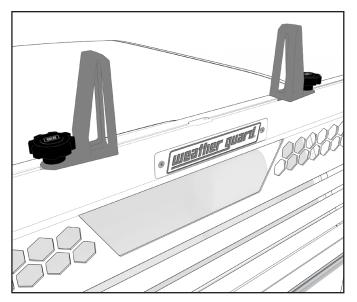
Position cargo stops along the top rail. Once in desired position, tighten using the knob.
