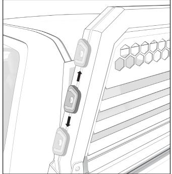
Position along rail to desired location. Tighten screw to secure.
