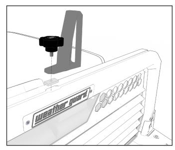
Using the knob to secure, insert the square nut into the slot. Loosely tighten the knob to the square nut.
