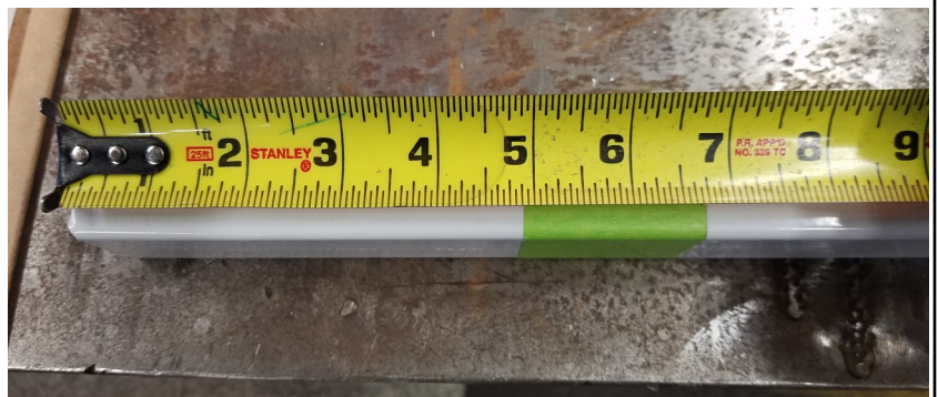
Proper taping of a Crossmember for directly mounting on a Ford Transit (4-7/8")
