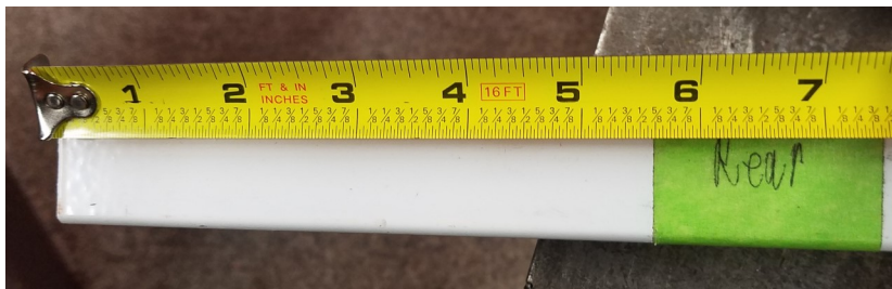
Proper taping of a rear Crossmember (5-5/8")
