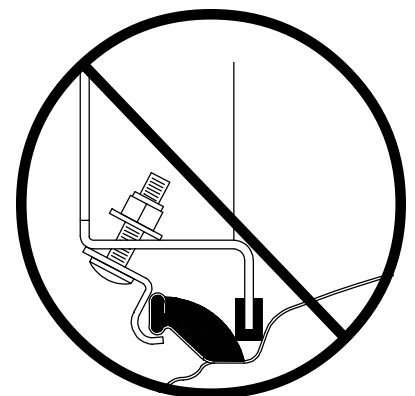
Figure 8. Example of unacceptable mounting. Not enough engagement of clamp and Stand does not contact bottom of gutter.
