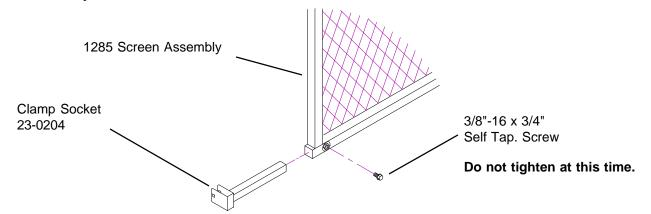
**Step 2.** Frame to Rack Assembly. Center screen between the ladder rack legs.
