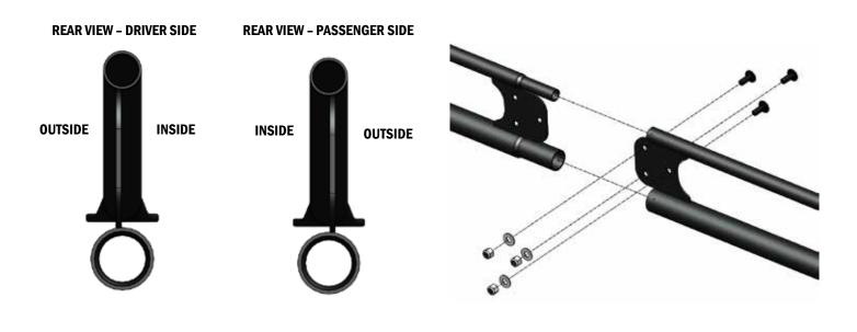
**STEP 4** Install the rear leg, with the tie down facing the outside using (1) Part C, (1) Part L, and (1) Part F. The outside plate will have the Weather Guard<sup>®</sup> logo.
