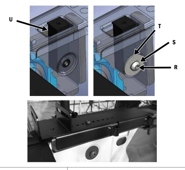
**STEP 14** Apply the rubber protective strip to the top of each of the cross members.
