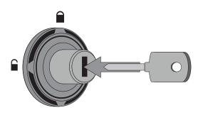
Turn key counter-clockwise 1/4 turn to unlock.
