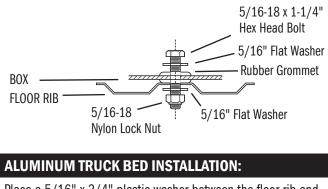
Place a  $5/16" \times 3/4"$  plastic washer between the floor rib and 5/16" flat washer. Place another  $5/16" \times 3/4"$  plastic washer between the rubber grommet and floor rib.
