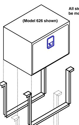
All steel and aluminum boxes must be mounted with either Type "A" or Type "B" brackets
