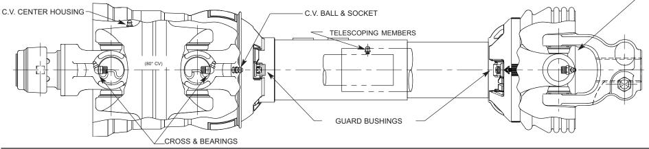
LUBRICATE ALL FITTINGS WITH A GOOD QUALITY LITHIUM SOAP COMPATIBLE E.P. GREASE MEETING THE N.L.G.I. #2 SPECIFICATIONS AND CONTAINING NO MORE THAN 1% MOLYBDENUM DISULFIDE.
