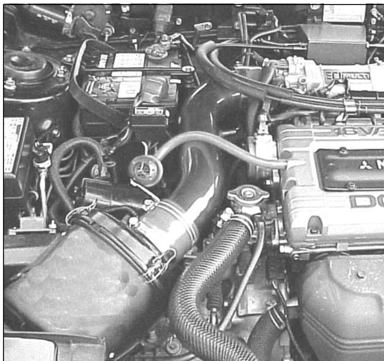
Intake install with filter insert inside enclosed OEM canister
