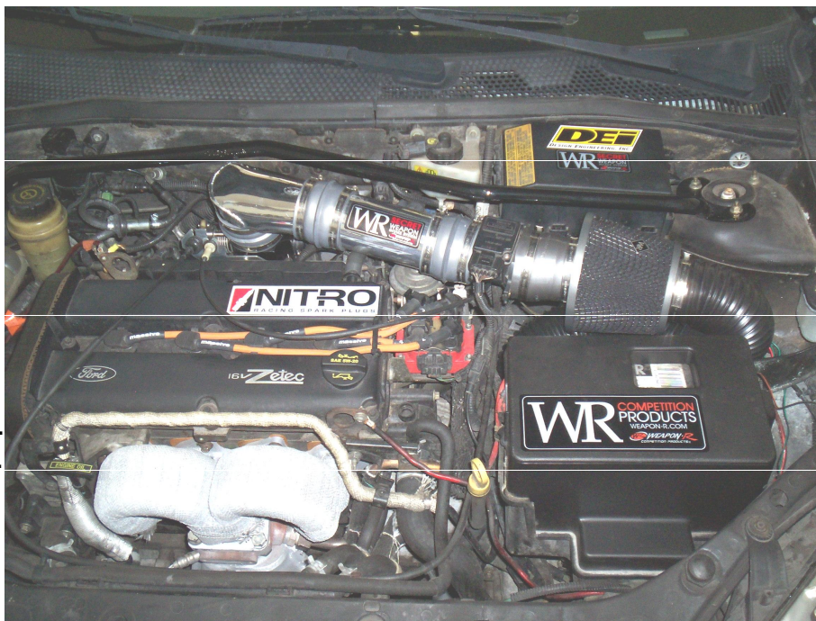
SW Intake install with Ram Air Kit II as shown. 2001 Focus ZX3 2.0L Ztec installation on picture.
