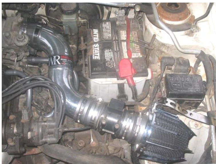
1996 Ford Escort GT 1.8L DOHC Dragon intake installed
