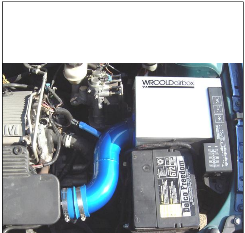
Intake with enclosed aluminum air box installed.
