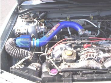
Dragon intake installed inside Aluminum air box ( flexi glass top cover upgrade not show ) Ram air kit install shown on top pic.
