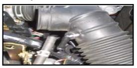
2 Unbolt MAF sensor from OEM air box. Set sensor aside for later steps. Wipe inside of throttle body clean of any oil residue or dirt. Take 3"-3" coupler and secure it onto throttle body with OEM clamp. Insert Weapon\*R intake pipe into coupler, and secure with supplied clamp.
