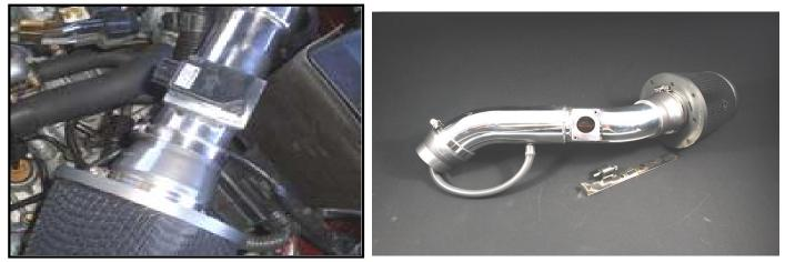
4 Check all clamps and connections for leaks, and clearances around intake before driving. Allow engine computer to adjust for at least 5 minutes before any high revving of engine
